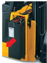
Battery removal CTX
